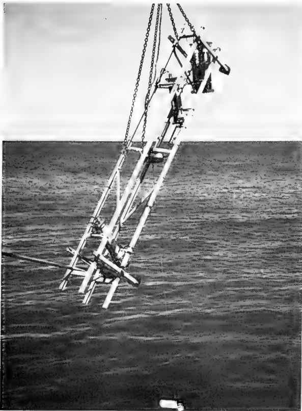
Figure 4. Special deep sea camera used by Woods Hole Oceanographic Institution from the Research Vessel Chain for photographing the Puerto Rican Trench at a depth of 20,000 feet. The camera features F-4.5 lens stereo cameras mounted side by side at the top of the framework, two electronic light sources mounted at the bottom of the framework and a sonar pinger for positioning the camera. The framework originally was designed in 1960 by Edgerton, Gernsmaier & Grier, Inc. for the U.S. Navy Hydrographic Office.
