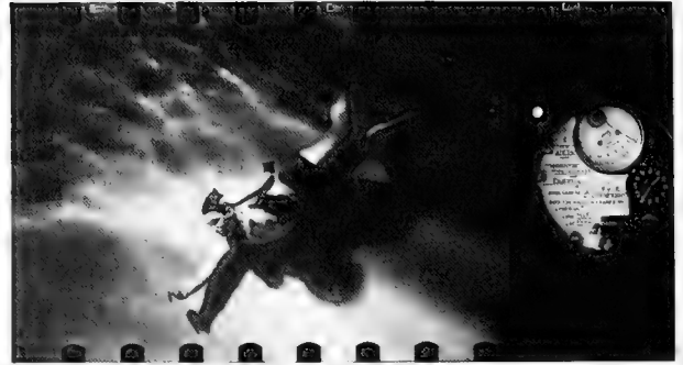
Figure 3. A photograph taken using the new Hopkins F-4.5 underwater lens. Compare the parallelism of the tile lines with those in Figure 2. The "data chamber" on the right is an internal part of the camera and records, date, time, and depth of each picture. The "data chamber" in the camera has been found to be invaluable in preventing the accidental switching of films. A small photo is taken with each photograph of pressure (depth), time on a 24-hour basis, and written in longitude and latitude information as well as the ship, date, etc.
