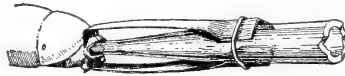
FIGURE 12.—Tip of drawn glass tubing, showing clips holding larva in place for inflation.
