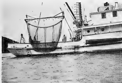
FIG. 16 - HOISTING THE BEAM TRAWL ABOARD THE JOHN N. COBB .
