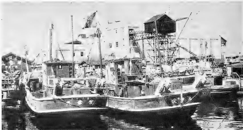
BULL TRAWLERS USED BY JAPANESE FISHERMEN IN THE EAST CHINA SEA. OPERATED IN PAIRS. FUKUOKA, KYUSHU, JAPAN.
