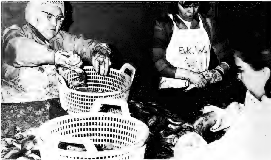
Fig. 2 - Herring roe is removed from the "aged" herring by first breaking the fish just behind the head, then using a squeeze-shake action to extract the roe from the carcass (woman on left). The ripeness of fish when caught is critical because seasonal maturity greatly influences both processing efficiency in removing roe and final quality of roe product. The amount of roe recovered from amount of herring landed is 8% to 10% by weight.
