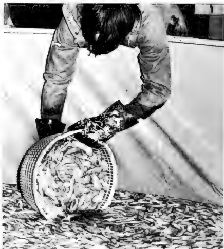
Fig. 4 - Basket of herring roe is put into a brine solution. During processing, roe is placed for 12 hours in each of three different brine solutions with a 3- to 6-hour drain period between each soak. The first two solutions have a salt content equivalent to sea water, the last a 100% solution of salt.
