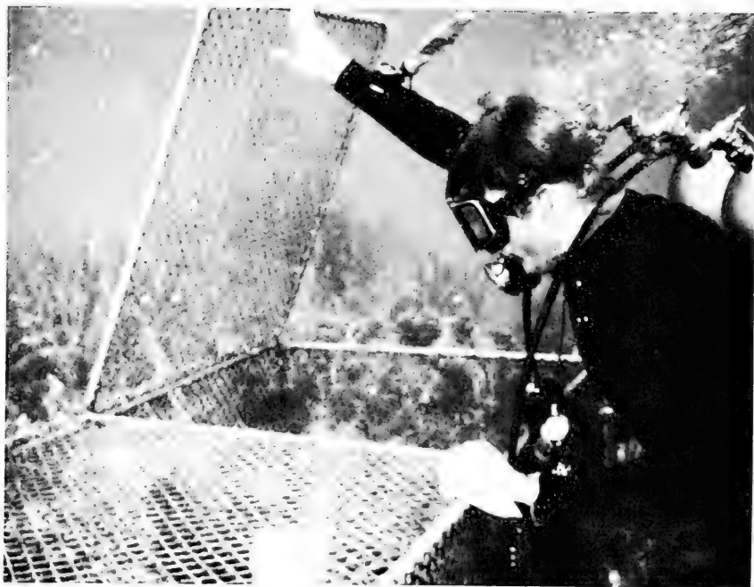
Fig. 4 - Underwater view of experimental pot lid opened to release captured fish.
