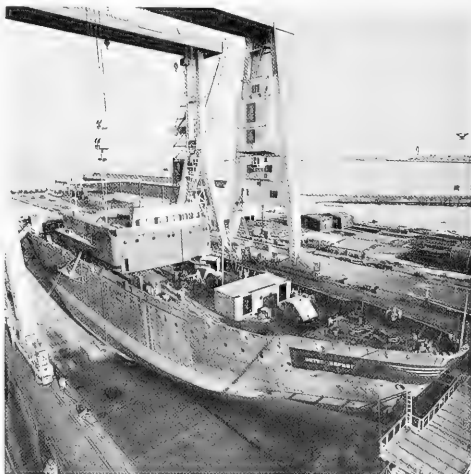
Fig. 1 - The M/S Vitus Bering , fish-freezing vessel built in Denmark for the U. S. S. R. Shows vessel almost completed on 19th working day.
