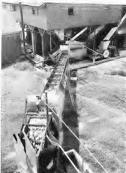
Fig. 2 - At an industrial fishery products plant in Moss Point, Miss., raw menhaden are being carried on a belt into the plant. Fish are carried either directly to a cooker or to temporary storage in raw box.
