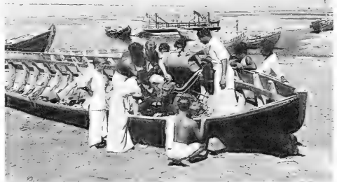
Fig. 2 - A Food and Agriculture Organization (FAO) expert installed two motors on two Ceylonese craft to demonstrate how the local boats could be motorized to advantage.
