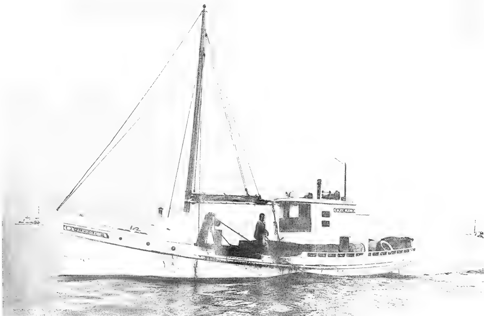
Fig. 9 - Dredge boats, often Diesel-propelled, are from 32 to 60 feet in length, five net tons or more, and tow two dredges simultaneously from opposite sides.
