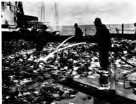
Fig. 4 - Washing silt and dirt from net loads of trawl-caught fish on the main deck of a typical Japanese factoryship.
