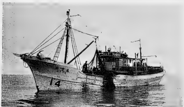
Fig. 1 - Typical small otter trawler fishing in the Bering Sea for a mothership.
