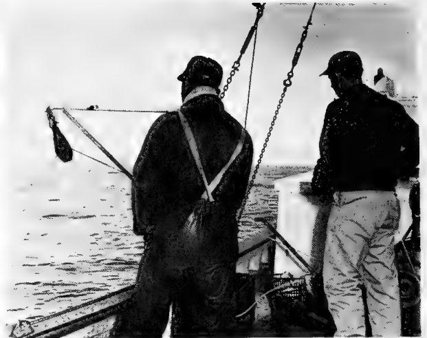
Fig. 2 - Hauling traps with a small davit and open block.
