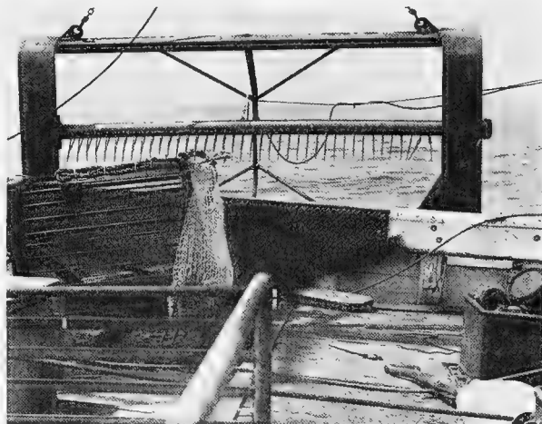
Fig. 4 - Clam sounder (at rail of vessel) used during survey operations. Note "teeth" mounted on pipe. Telephone microphones which transmit the sounds of clams being struck by the teeth are secured inside the pipe.
