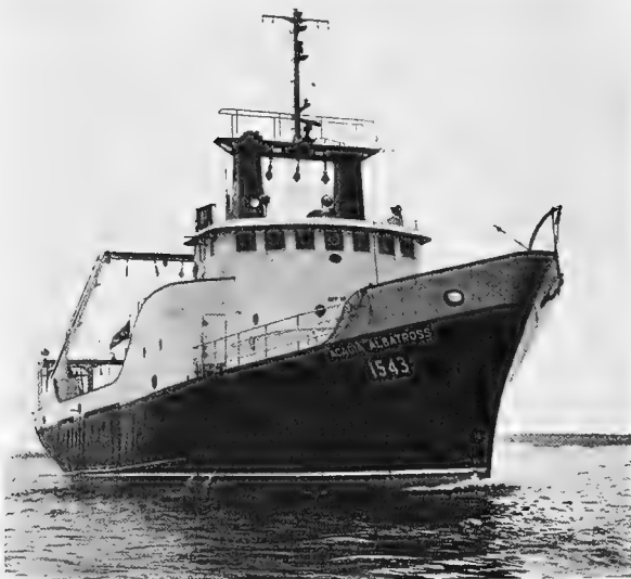
Fig. 2 - The Acadia Albatross , a modern Canadian stern trawler. The vessel, all-welded steel strengthened for navigation in ice, is 152 feet long overall. Vessel is operated by a Nova Scotia fisheries firm.
