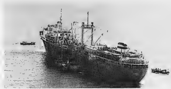
Fig. 10 - Zakharov -class factoryship operating in the king crab fishery of the eastern Bering Sea. In the shadow of the vessel is an SRT trawler. Factoryship carries 12 motorboats for king crab fishing - one is near the bow and another near the stern.
