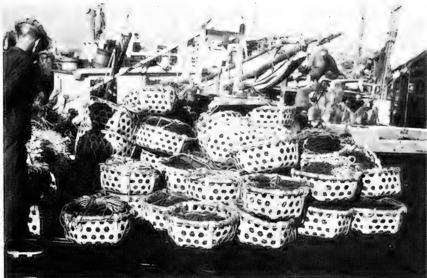
FIGURE 8 - BASKETS OF LONG-LINE GEAR READY TO BE STOWED ABOARD VESSEL. EACH BASKET CONTAINS FLOAT, MAIN, AND BRANCH LINES (INCLUDING HOOKS) ARRANGED IN PROPER SEQUENCE FOR RAPID HANDLING DURING THE SETTING-OUT OPERATION.
