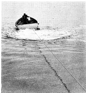
FIG. 9 - THE SKIFF TOWS THE VESSEL AWAY FROM THE SEINE DURING PURSING AND HAULING
