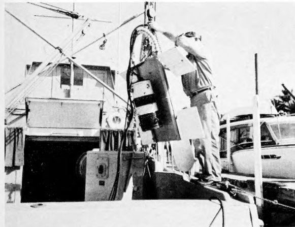
Fig. 5 - Camera housing mounted on sled for rear viewing.
