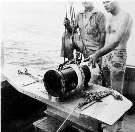
Fig. 3 - Early experimental mounting of TV housing on submersible sled, Camera set for side viewing.
