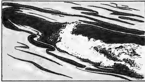
FIG. 3 - HYDRODYNAMIC TESTS OF ORIGINAL TRAWL PLANE FLOAT REVEALED THAT THE DRAG FACTOR WAS EXCESSIVE AND OVERCAME UPTHRUST AT SPEEDS OF TOW ABOVE 3 KNOTS. SKETCH SHOWS VORTEX CREATED BY DRAG IN THE ORIGINAL MODEL OF THE WEIGHTED PLANE BEING TOWED IN A SWIMMING POOL.
