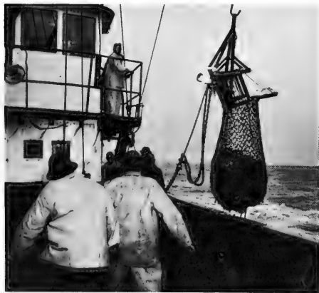
Fig. 1 - Commercial catch ( 6\frac{1}{2} bushels) of hard clams ( Venus sp.) taken by the Silver Bay off Beaufort, N. C., in 6 fathoms. The chain bridle and the accumulator can be seen.
