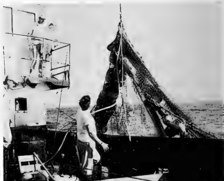
Fig. 8 - Bosom rollers being brought on deck with the "gilson" (whip). Wing rollers remain overboard.
