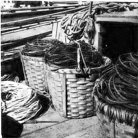
Fig. 6 - Long-line gear aboard the Aries out of Gloucester, Mass. Three baskets are fished to make a 750-fathom main line with 150 hooks. Note rubber mackerel lure on center basket.
