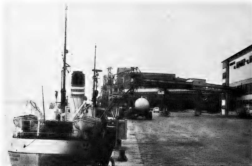
Fig. 4 - German distant-water trawler tied up at dock, Hamburg. Note overhead ice conveyor for icing-up vessels.
