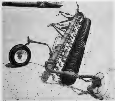
Fig. 1 - A type of underwater harrow used as a mechanical method of control of oyster enemies.
