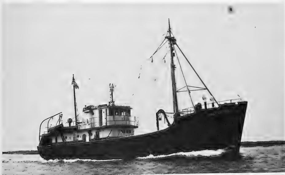
Fig. 1 - The M/V Silver Bay --96.4-foot North Atlantic dragger used in the snapper-trawl studies.
