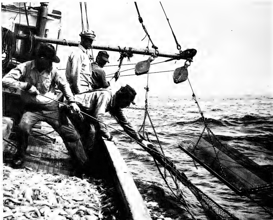
Shrimp trawling in Gulf of Mexico off New Orleans. Trawl and otter boards, suspended from outrigger boom, are being lowered back to fish again. Part of last mixed catch of fish and shrimp is on deck. (C.H.B.)
