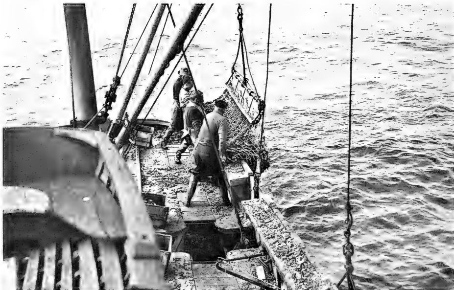
Fig. 2 - Dredge nets are used on New Zealand oyster boats that fish out of Bluff harbor into Foveaux Strait. Here a net is being swung inboard, and the catch tipped onto a culching bench for sorting. (Culching is separating the shells of takable size, believed to contain oysters, from material dredged from bottom.)
