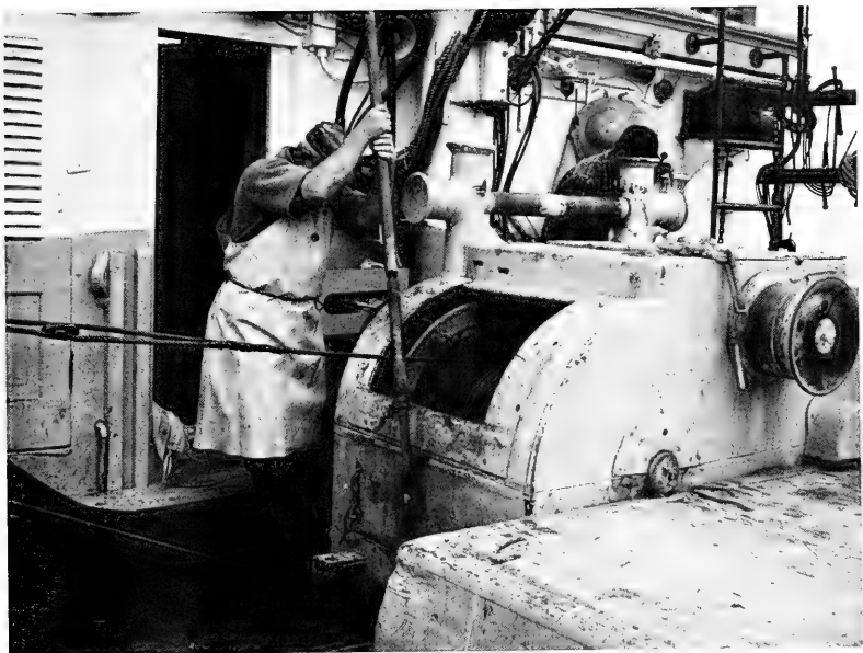
Fig. 18 - Modified dragger winch being used to purse the net.
