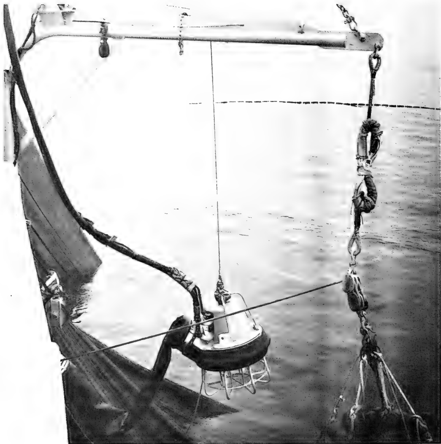
Fig. 5 - Capsul-pump attached to "Morgan" boom.
