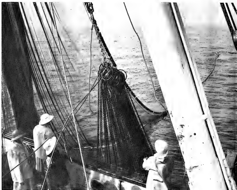
Fig. 14 - Purse rings being hoisted on deck.
