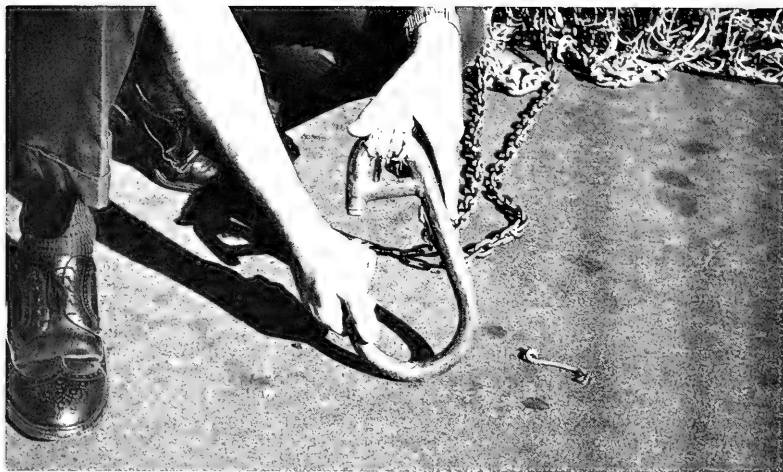
Fig. 13 - Snap ring in open position.
