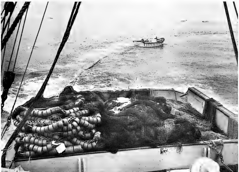
Fig. 8 - Net skiff being used at the start of a set.
