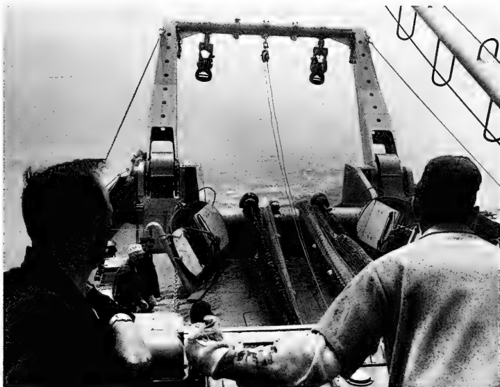
Crew of NMFS research vessel 'Albatross IV' retrieves fishery gear off Georges Banks during experimental fishing operations. Vessel has stern trawling ramp, bow thruster to help control it on station, variable pitch propeller, active rudder and closed circuit television. TV shows operations on vessel and trawl and other gear.
