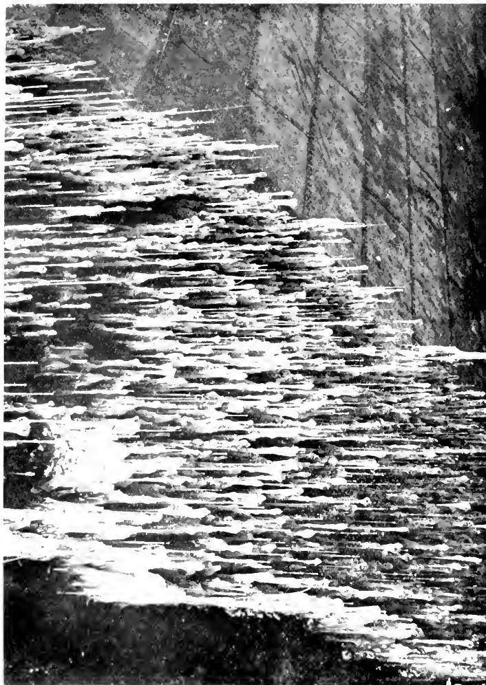
CONDITION BELOW THE WATER-LINE OF THE HULL OF U.S.S. "FERRIE" WHEN DOCKED, GREATLY REDUCING THE SPEED WHICH SHOULD HAVE BEEN DERIVED
