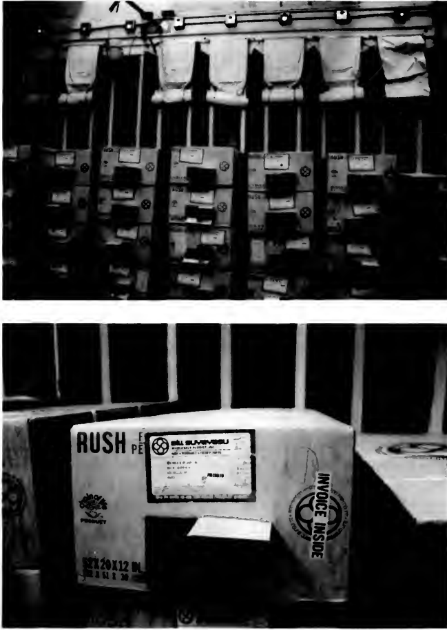
Figure 6-1. A Pre-cooler in Operation and a Close-up of the Built-in Portholes in the Boxes (Cold air is pulled through the boxes from the surrounding refrigerated atmosphere.)
