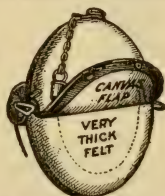
Sectional View of Water Cooling Canteen.
