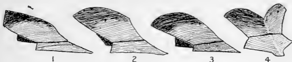
FIG. 77. Four types of plows: 1, a breaker. 2, a general-purpose plow for use in light land. 3, a black-land plow. 4, a middle burster.
