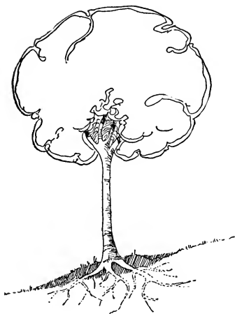
Fig. 10.—If, in grading, the general level is lowered where valuable trees stand, gentle mounds should be left around and over the roots of such specimens as shown here in cross section
