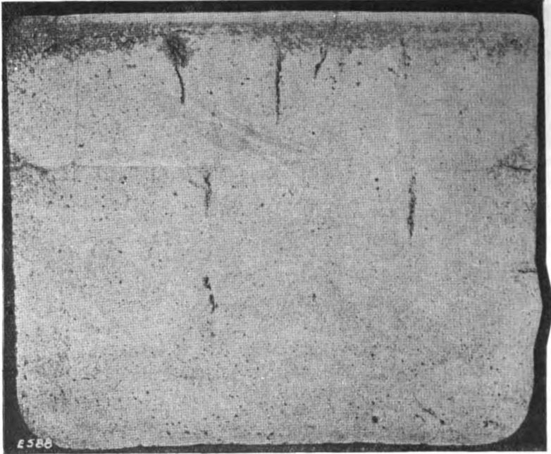
FIG. 4. Unhydrated Cement and Gradation of Particles from top to bottom are found in this Year-old Block of Neat Cement.
