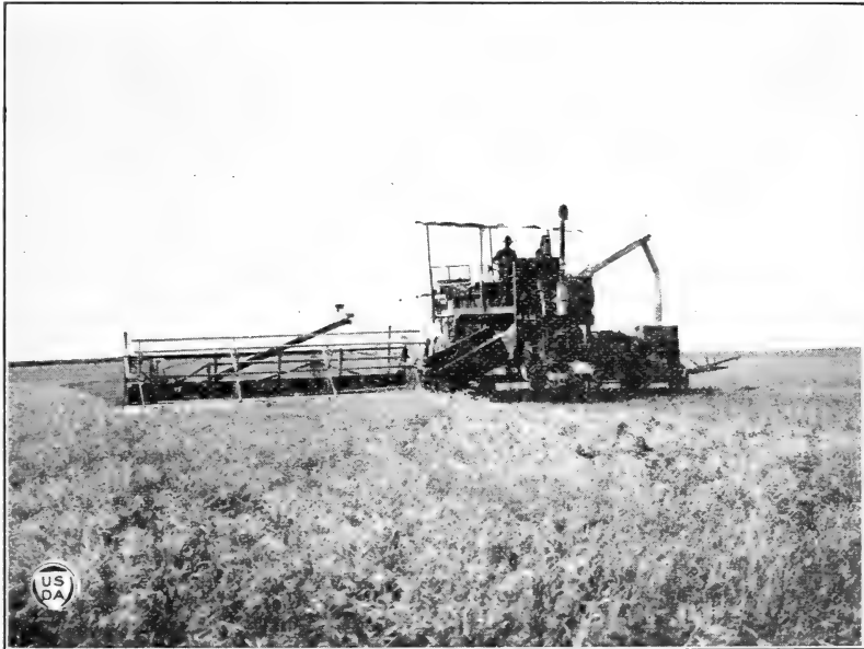
FIG. 5.—Front view of a combine. The grain chute extends to the right, with the grain running out into the grain barge. This combine furnished traction for itself and for the grain barge. When full, the barge is hauled away by a team and another empty barge is substituted. One teamster and a team are thus kept busy hauling. This method of harvesting and threshing reduces the use of man and horse power to a minimum.
