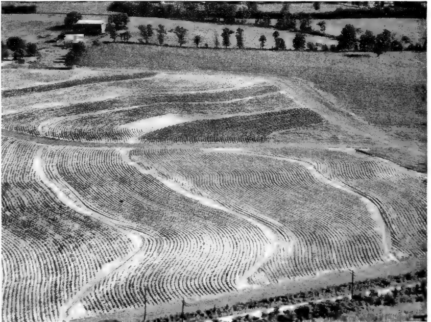
FIGURE 19.—A well-planned tobacco field in southern Maryland, which includes terraces, grassed terrace outlets, and ridged rows. The guide rows in this field were located by the string method to give effective erosion control and adequate drainage.
