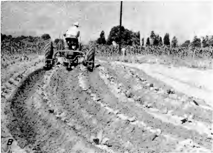
FIGURE 22.—On this southern Maryland farm both the planting and cultivation of tobacco is done by machinery. A , Planting tobacco on ridged rows with a two-row tractor planter on the H. W. Townshend farm. B , Cultivating ridged tobacco with two-row tractor cultivator proved satisfactory on this farm.
