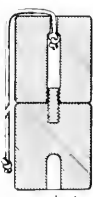
Fig. 57. Weight and cord. The weight unscrews in the middle, the connector pin remaining with the lower half.
