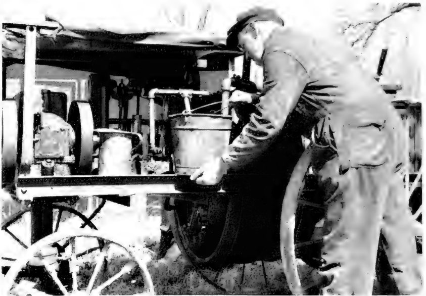
Fig. 3.—Mixing spray material by the injector method.
