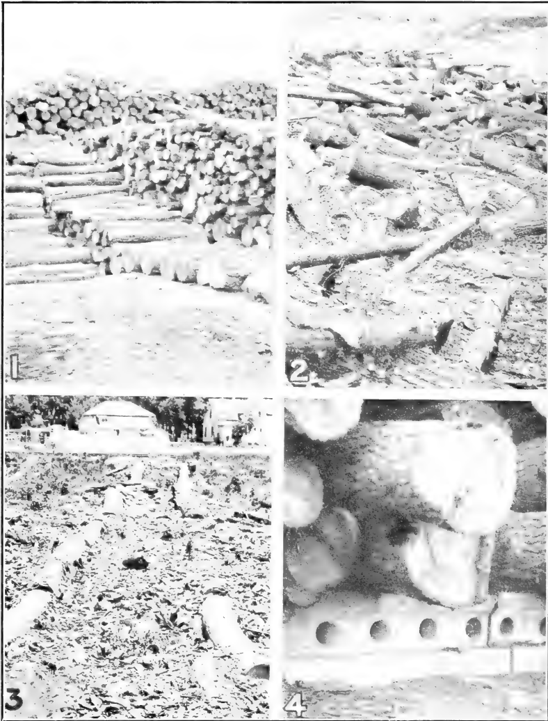
FIG. 1.—Four-foot hemlock piled directly on the ground and with no spacing between the ranks. Wood should never be placed directly on the ground. Even if these ranks had been separated, the pile in the background running at right angles to them would have cut off most of the air circulation.
