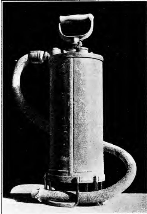
Fig. 2.—Karbo-Killer, for pumping carbon bisulfide into rodent burrows.
