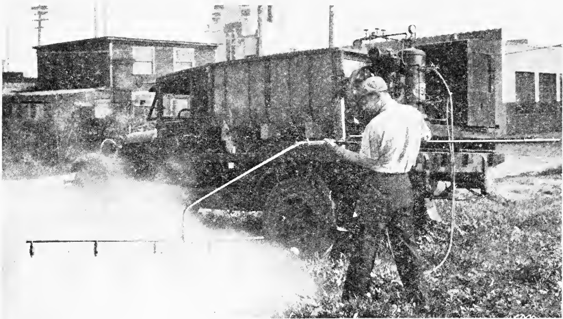
Fig. 7.—Power rig equipped with two lines—one air, one liquid—which produces atomization, thus giving a very even and thin coverage. This machine shows lines attached to multiple nozzle.
