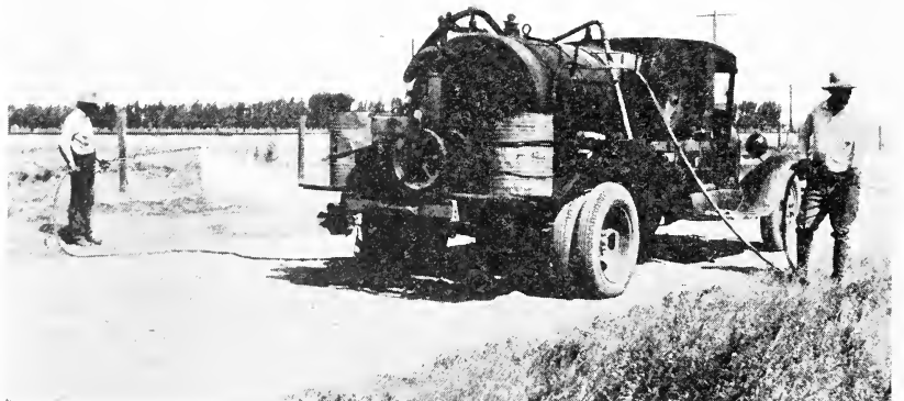
Fig. 6.—Power spray equipment adapted for spot work along roads. Two lines of hose.
