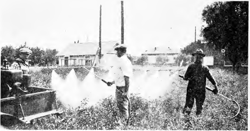
Fig. 4.—Power spray rig, showing two lines of hose with multiple nozzle.
