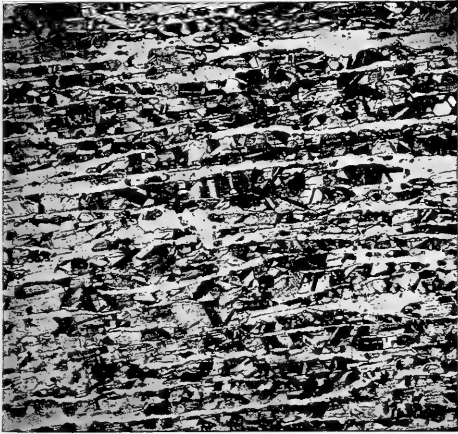
Fig. 1.—Hot-rolled Roman-bronze shafting rod (longitudinal section). Etchant \text{NH}_4\text{OH} + \text{H}_2\text{O}_2 . 75 \times
