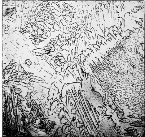
Fig. 2.—Extruded naval-brass rod (longitudinal section). Etchant \text{NH}_4\text{OH} + \text{H}_2\text{O}_2 . 75 \times
