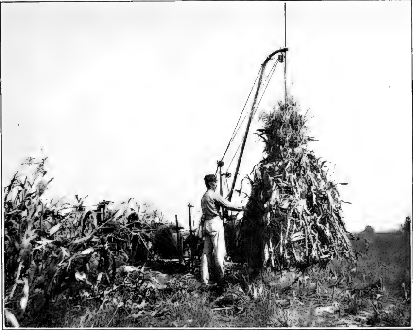
FIG. 1.—CORN SHOCKER UNLOADING THE SHOCK.
