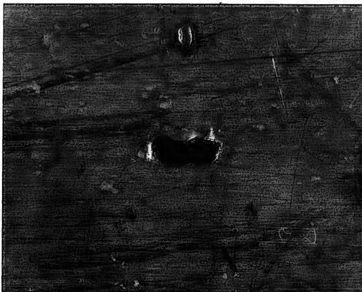
Figure 3. Typical pitting corrosion in stainless steel.
