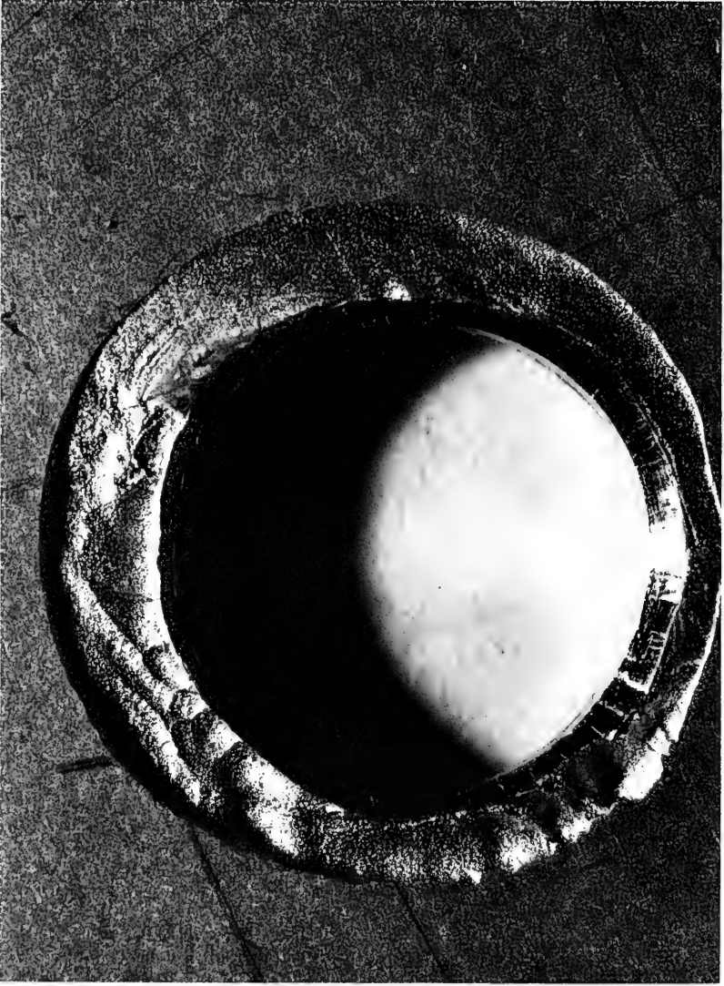
Figure 5. Crevice corrosion typical of that found in stainless steels.
