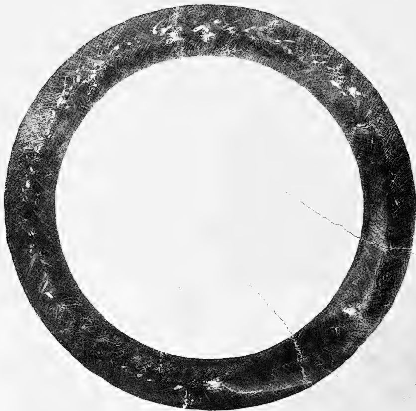
Figure 14. Stress corrosion cracks in circular welded 13V-11Cr-3Al alloy after 181 days of exposure in surface sea water.
