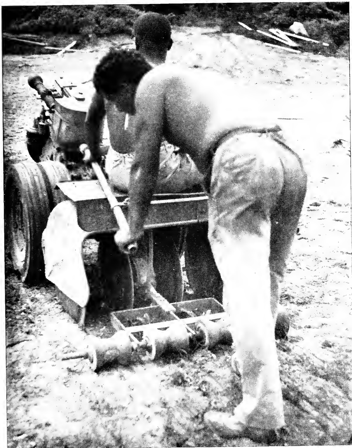
Vine setter, developed by "Bob" Pierce (page 10), showing disks and rollers.
