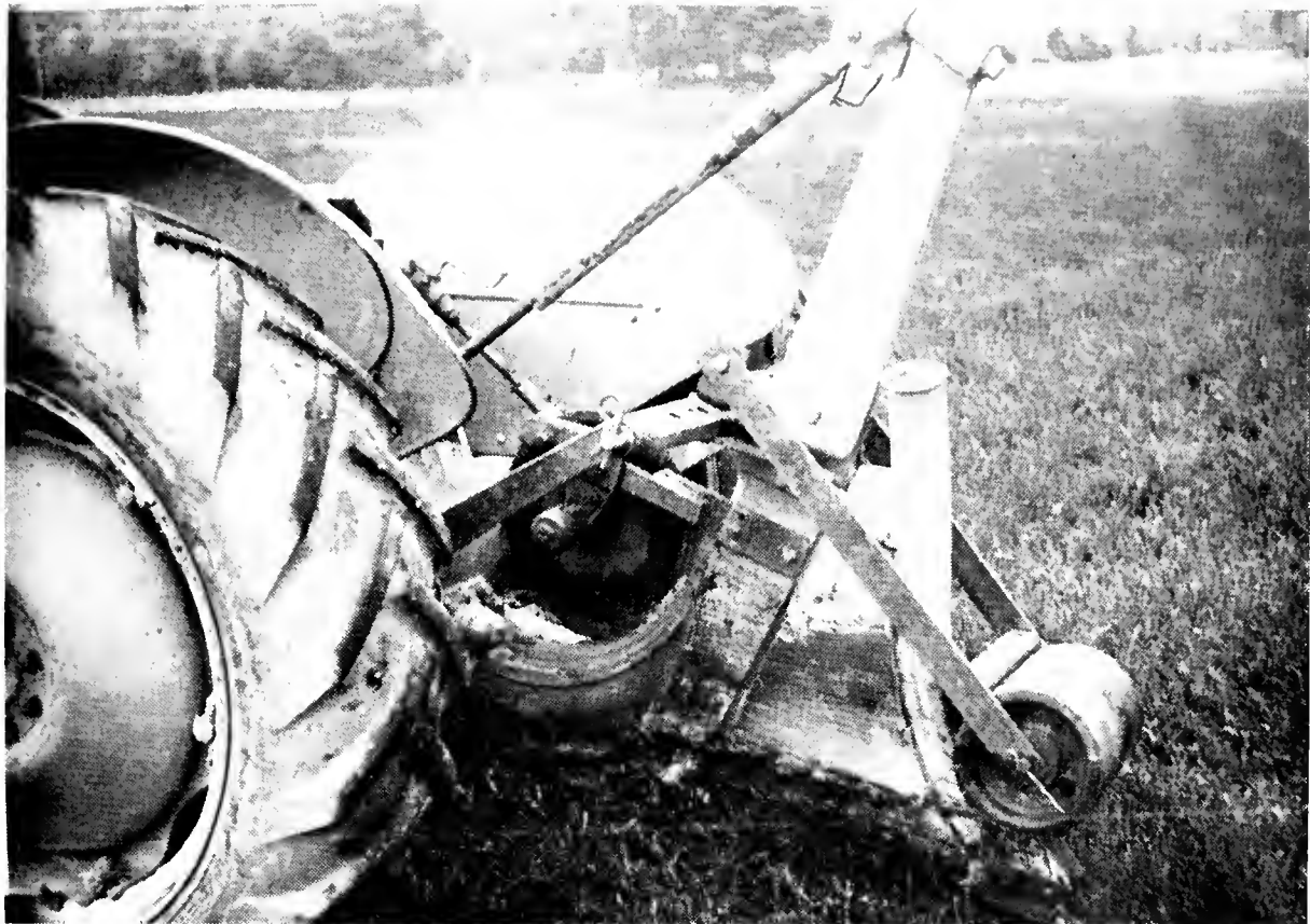
Plow attachment for the installation of polyethelene drainage tubing is shown here. Tube is fed through the pipe near the rear of the attachment and the roller, right, smooths down the turf after the pipe has been inserted. (Photo by F. B. Chandler)
