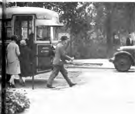
Old No. 1 pioneered CSL's bus service on Aug. 10, 1927, working the Diversey Extension with no backup unit available until four more buses arrived weeks later. In view looking south at Diversey-Cicero, note brick-paved intersection and concrete curb lanes with dirt center strip reserved for streetcar tracks.
