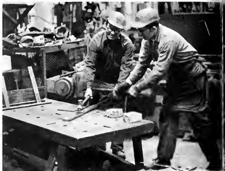
John Maros, shopman II, (left) pounds the reshaped fish plate with a sledgehammer as part of the finishing touches.
