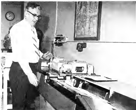
Leonard Skrine, supervisor of the CTA mail room, is shown at one of the two metering machines which, when working at capacity, can stamp 375 envelopes per minute.
