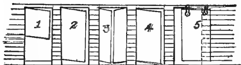
FIG. 63.—Methods of hanging doors. 1, The upper half swings out; 2, the door swings both ways on a two-way hinge; 3, each half swings out; 4, the door swings out; 5, the door slides to one side on a track.
