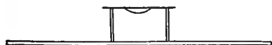
FIG. 2. Van Tieghem cell for work with hanging drop, as seen in section
