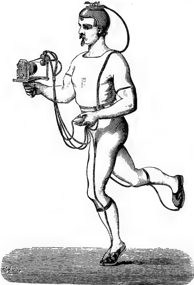
FIG. 494.—Runner provided with apparatus intended to register his different paces (Marey).
