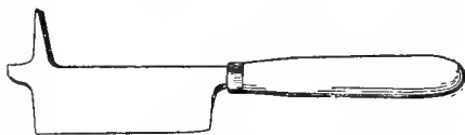
FIG. 115. — Grafting chisel for making the cleft in cleft-grafting. The point at the left is for holding the cleft open during insertion of cions. The projection above is for driving this point in or out; one-fifth natural size.
