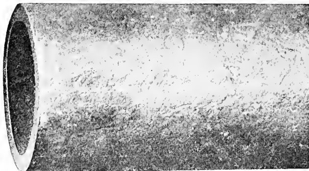
FIG. 6.—PIPE USED FOR FOUR YEARS WITH CALCIUM CHLORIDE.
