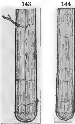
FIGS. 143-144. — Diagrams of tree trunks, showing knots of different ages: 143, from tree grown in the open; 144, from tree grown in a dense forest.
