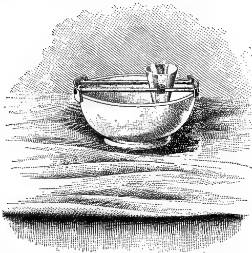
FIG. 235. BOWL WITH DRAINING RACK AND FUNNEL FOR STAINING SECTIONS.
