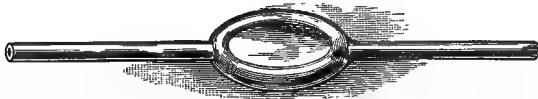
Fig. 12.—One of Brefeld's " kammer " for nährlösung cultures. It consists of a glass tube open at both ends; in the middle a bulb has been blown which has been compressed laterally, so that its sides are parallel to each other, or nearly so. When in use the two open ends of the tube are closed with cotton wool.
