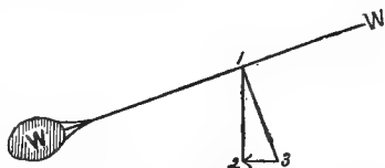
FIG. 316.—Cross section of the wing plane of a bird, showing its action in flying.
