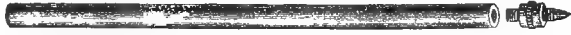
FIG. 136. Writing diamond for writing numbers and labels on glass slides, cutting cover-glasses, etc. (Queen & Co.).
