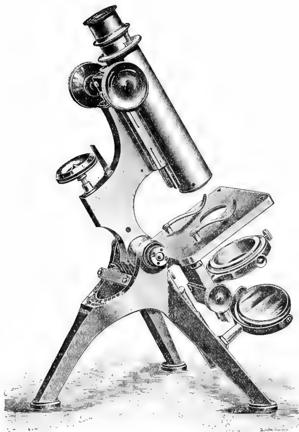
FIG. 71. Watson & Sons' Edinburgh Students' Microscope (Stand G). This is a good representative of the tripod-base, English models of to-day. It is in general like the Powell and Lealand stands which have held their position with the foremost English microscopists for the last 40 years. (See Carpenter-Dallinger, p. 172).
