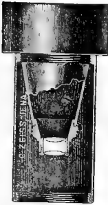
FIG. 149. Zeiss' Apochromatic, Projection Objective of 70 mm. equivalent focus, for photo-micrography. (Zeiss' Catalog. No. 30), This, and another of 35 mm. focus, are designed for making pictures of moderate magnification. Usually rather large objects are photographed with them. The object may be illuminated in the ordinary way. They are used without an ocular, like a photographic objective. The one of 35 mm. is screwed into the tube of the microscope like an ordinary objective, but the one of 70 mm. here shown, is, by means of a conical adapter, screwed into the ocular end of the tube.
