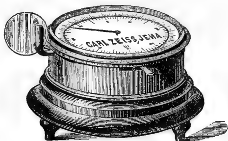
FIG. 122. Zeiss Cover-Glass Measurer. With this the knife edge jaws are opened by means of a lever, and the cover inserted. The thickness may then be read off on the face as the pointer indicates the thickness in hundredths millimeter in the outer circle and in hundredths inch on the inner circle.
