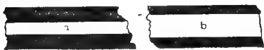
FIG. 89. Solid glass rod showing the appearance when viewed with transmitted, central light, and with an objective of medium aperture.
