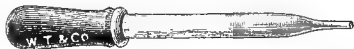
FIG. 133. Pipette for adding liquids dropwise and for washing preparations. (Whitall, Tatum & Co.)
