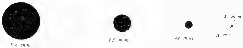
FIG. 37. Figures showing approximately the actual size of the field with objectives of 85 mm., 45 mm., 17 mm., 5 mm., and 2 mm., equivalent focus, and ocular of 37\frac{1}{2} mm., equivalent focus in each case. This figure shows graphically what is also very clearly indicated in the table (§ 52).
