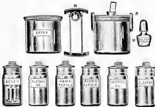
FIG. 160. Apparatus and reagents with which the slide holders are used. With this apparatus it is easy to prepare specimens in large numbers very expeditiously. After the sections are fastened to the slide and placed in the holder, the slides need not be touched during all the operations until they are finally ready to be mounted in balsam. Each holder contains from 12 to 14 slides. (§ 277-300). The bottles for the reagents are glass stoppered specimen or museum bottles. (Mix, Jour. Ap. Micr. 1898, p. 171.) Compare Fig. 148.
