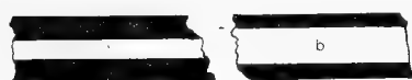
FIG. 92. Solid glass rod showing the appearance when viewed with transmitted, central light, and with an objective of medium aperture.
