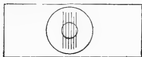
FIG. 96. Diagram of a stage micrometer, with a ring on the lines to facilitate finding them.
