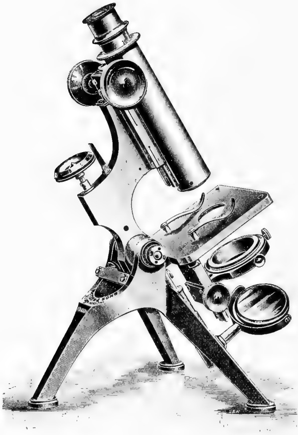
FIG. 85. Watson & Sons, Edinburgh Students' Microscope (Stand G). This is a good representative of the tripod-base, English models of to-day. It is in general like the Powell and Lealand stands which have held their position with the foremost English microscopists for the last 40 years. (See Carpenter-Dallinger, p. 172.)
