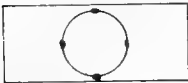
FIG. 139. Slide and cover-glass showing method of anchoring a cover-glass with a glycerin preparation when no cell is used. A cover-glass so anchored is not liable to move when the cover is being sealed (§ 253).
