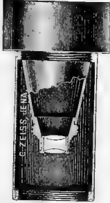
FIG. 183. Zeiss' Apochromatic Projection Objective of 70 mm. equivalent focus, for photo-micrography. (Zeiss' Catalog.)
