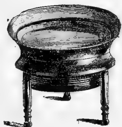
Fig 164. Tripod magnifier as a focusing glass. This is carefully focused on a scratch or pencil mark on the lower or ground surface of the focusing screen. Then whenever the object is sharply focused the focal plane will be at the level of the sensitive surface.
