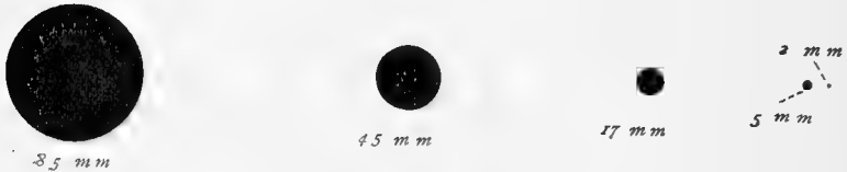
FIG. 42. Figures showing approximately the actual size of the field with objectives of 85 mm., 45 mm., 17 mm., 5 mm. and 2 mm., equivalent focus, and an ocular of 37\frac{1}{2} mm. equivalent focus in each case. This figure shows graphically what is also very clearly indicated in the table (§ 59).
