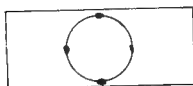
FIG. 200. Slide and cover-glass showing method of anchoring a cover-glass with a glycerin preparation when no cell is used. A cover-glass so anchored is not liable to move when the cover is being sealed (§ 351).
