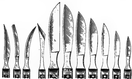
FIG. 232. Various forms of scalpels. The one at the left is especially excellent for cutting the ribbons of sections of the proper length for mounting. The large one with straight edge is the best form for trimming the paraffin block square for sectioning. (Cut loaned by the Bausch & Lomb Optical Co.)
