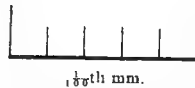
FIG. 131. Showing the method of indicating the scale at which a drawing was made.
