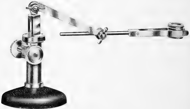
FIG. 113. Simple microscope mechanically supported by a lens holder. One may obtain the magnifying power of a simple microscope by the use of a camera lucida as with the compound microscope. (Cut loaned by the Spencer Lens Co.)
