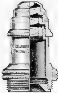
FIG. 29. An objective in section, showing the different combinations formed of concave and convex lenses. Cut loaned by Voigtländer & Sohn, A. G.
