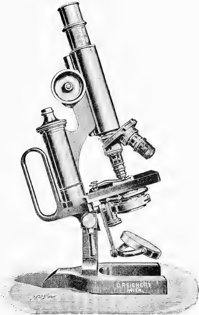
FIG. 88. Reichert's Laboratory Microscope with Handle. This handle is so attached that it does not preclude the ordinary means for fine adjustment.
