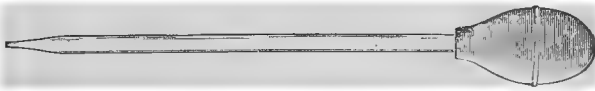
FIG. 250. Pipette with large rubber bulb for adding liquids to preparations. (Cut loaned by the Bausch & Lomb Optical Co.)
