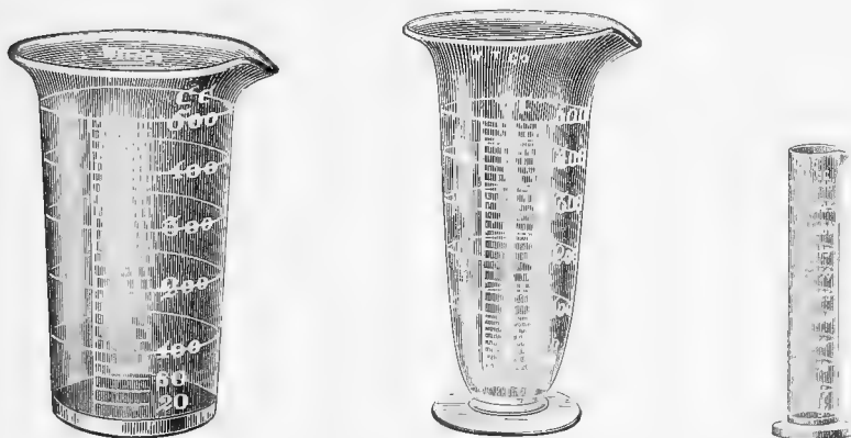
FIGS. 215-217. Graduates of various forms for measuring liquids. (Cuts loaned by the Whitall Tatum Co.)
