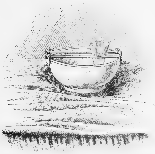
FIG. 248. Waste bowl with rack for supporting slides and a small funnel in which the slides stand while draining. This outfit is easily made by any tinsmith. The rack is composed of two brass rods about 4 mm. in diameter. The bent end pieces are sheet lead. The funnel is made of tin, copper or brass. Either copper or brass is preferable to tin. A glass dish like that shown in Figs. 188, 251 is better than a bowl, as it can be more readily and thoroughly cleaned. (Cut loaned by Wm Wood & Co.)
