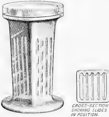
FIG. 252. Copley's staining dish. A. The entire dish; B. The dish in cross section. This is made of glass and is a very neat piece of apparatus. With it ten slides may be stained at once. (Cut loaned by the Whitall Tatum Co.)
