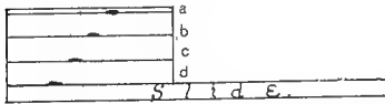
FIG. 96. Letters mounted in stairs to show the order of coming into focus.
