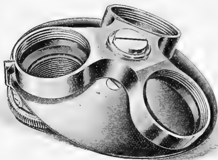
FIG. 40. Triple nose-piece or revolver for quickly changing objectives.
