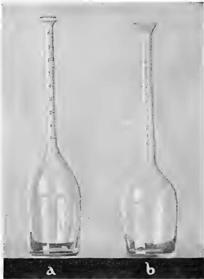
FIG. 104.—Milk test bottles. a is very much preferable to b . First, in having a slender neck, which will permit of accurate reading of the fat; second, in having sloping shoulders. Fat will lodge under the abrupt shoulder of b , and thus reduce the reading; third, the top of a is not flaring as b . A milk tested in duplicate in two bottles such as these would not read the same.
