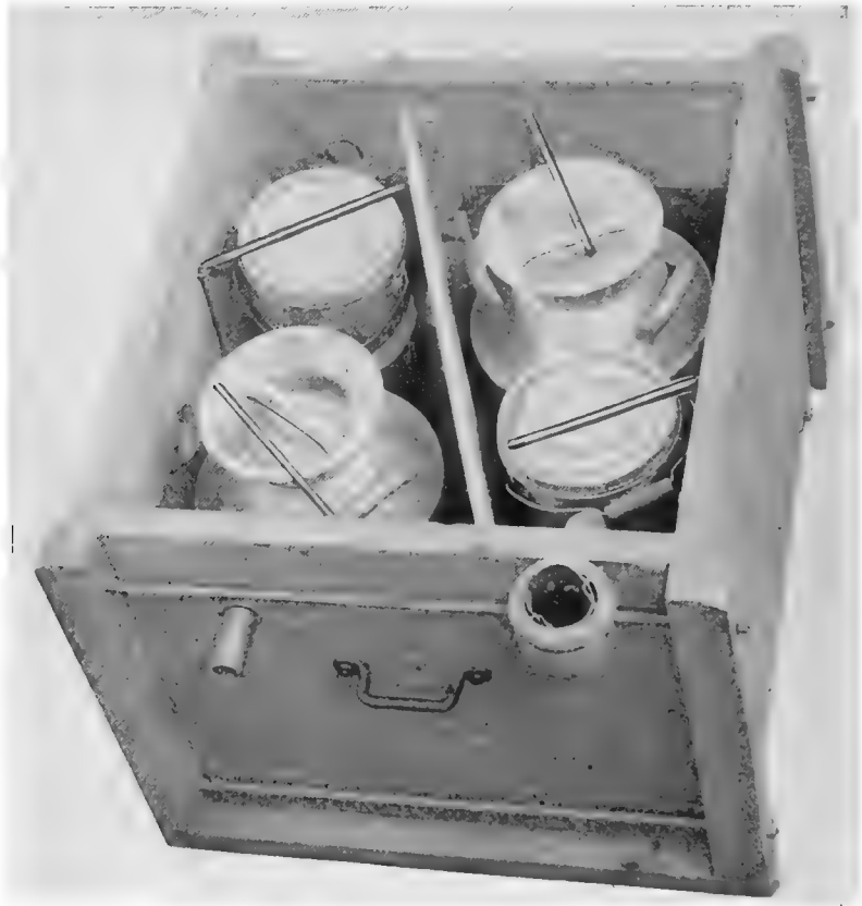
FIG. 113.—Milk cooling tank, cover off to show arrangement of cans. All water pumped for the stock passes first through this tank. (Courtesy Minnesota Tank and Silo Co., Minneapolis, Minn.)
