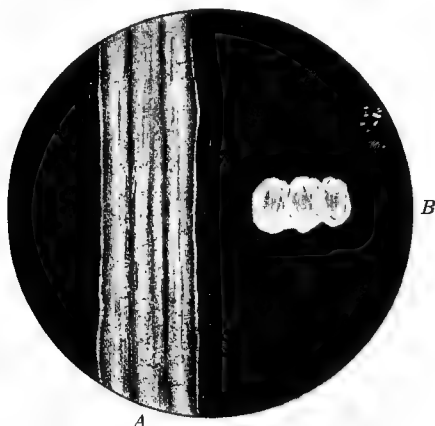
FIG. 197.—Kemp, structureless like fibers that are brittle and do not take the color dyes. A , longitudinal section, B , cross-section, compare with Fig. 24. (From "Structure the Wool Fiber," Bowman. Courtesy of The Macmillan Co.)
