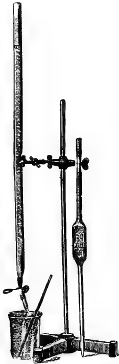
Fig. 28.—The Manns' acidimeter or acid test.
