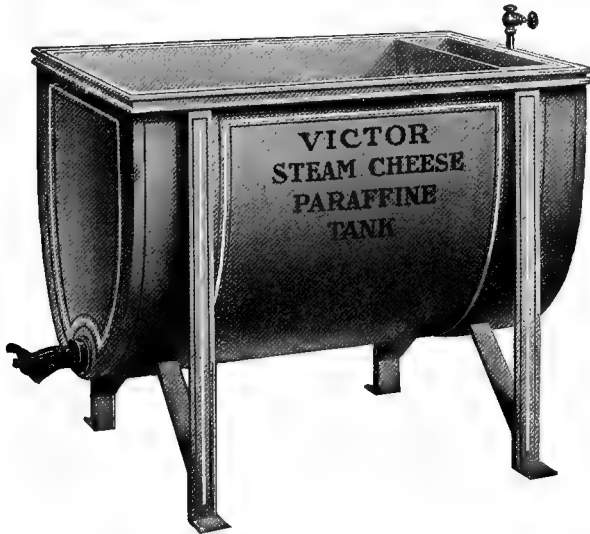
Fig. 54.—Tank used for paraffining Cheddar cheese in factories. The steam is admitted into the jacket around the tank and keeps the paraffine at the proper temperature. By means of such a tank and a pair of dipping tongs cheese can be paraffined easily and rapidly.
