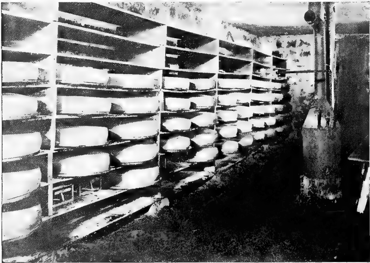
Fig. 76.—Curing cellar in a Swiss cheese factory, near Monroe, Wis. The large drum Swiss cheese are on the shelves. The small boiler supplies steam for moisture when too dry.
