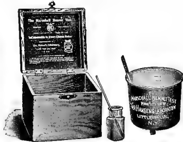
Fig. 21.—The Marschall Rennet Test. A, graduated cup; B, 1 c. c. pipette; C, glass in which to dilute the rennet; D, spatula for stirring the milk.
