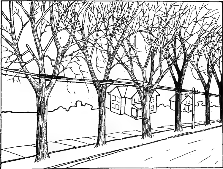
Fig. 13. The Same Trees as in Fig. 12, With Crowns Saved and Wires Carried Thru Them in Cables on Low Poles.
